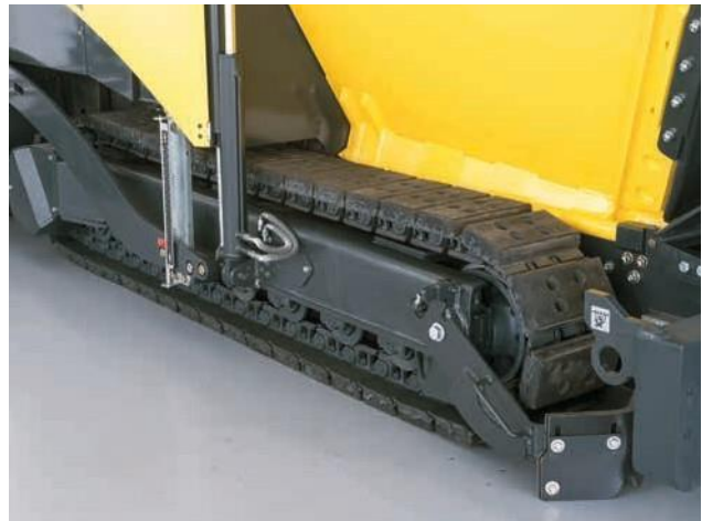
Long crawler tracks ensure dead straight paving.
